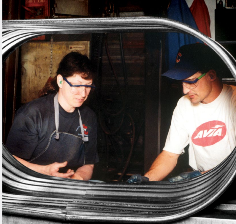
Two workers assemble a galvanized metal stock tank at Behlen Manufacturing in Columbus, Neb. Capacities of Behlen metal tanks range from 44 gallons to 1,117 gallons.
